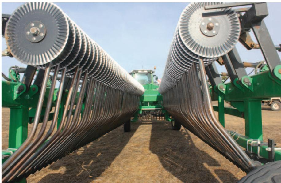
THE K-LINE TRASHCUTTER, SHOWN HERE FOLDED FOR TRANSPORT, IS DOING A GOOD JOB ON MEDIC VINE FOR DARYL NORRIS, THANKS IN PART TO THE EXTENDED FINGERS THAT PRESS RESIDUE ONTO THE SOIL SURFACE AHEAD OF THE RIPPLED COULTERS.
