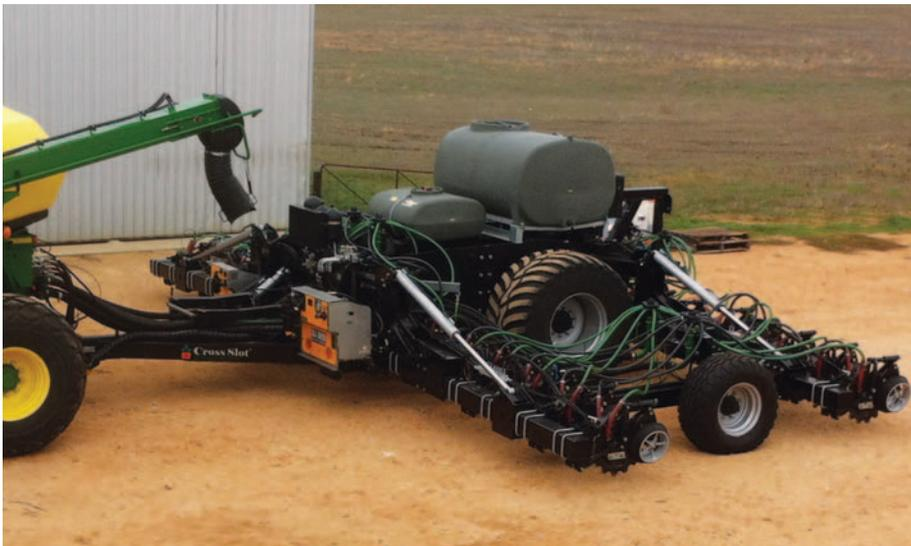
EACH SEEDING UNIT ON THE CROSS SLOT COMPRISES AN L-SHAPED BLADE ON EITHER SIDE OF A CENTRAL DISC THAT CUTS THROUGH SURFACE RESIDUE AND OPENS THE SEEDING SLOT. THIS PROVIDES GOOD CONTROL OF SEEDING DEPTH AND SEPARATION OF SEED AND FERTILISER, WITH MINIMAL DISTURBANCE OF THE SOIL SURFACE AND WITHOUT DISTURBING STONE IN THE SOIL.
