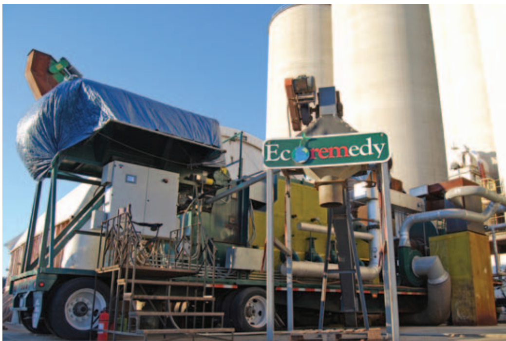
FIGURE 1. OPERATION OF AN ECOREMEDY® PILOT PLANT BEGAN IN MARCH OF 2008. THE FACILITY WAS LOCATED AT TYSON FOODS' FEED MILL IN FAIRMOUNT, GEORGIA. TYSON IS AMERICA'S LARGEST PRODUCER OF POULTRY MEAT. OVER THE COURSE OF 11 MONTHS THE PLANT OPERATED 24 HOURS A DAY, FIVE DAYS A WEEK, AND IN THAT TIME CONVERTED MORE THAN 500 TONS OF POULTRY LITTER TO ENERGY THAT WAS USED TO GENERATE STEAM FOR USE IN THE FEED MILL. THIS ALSO REDUCED METHANE EMISSIONS; A BENEFIT THAT OFFERS POTENTIAL FOR SIGNIFICANT REVENUE FROM THE CARBON ECONOMY.
