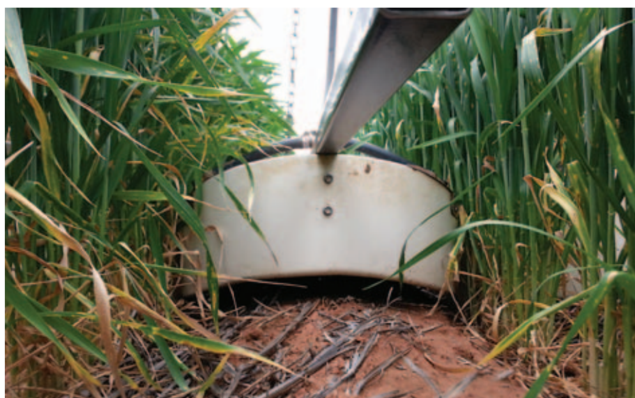
A CLOSE-UP OF ONE OF THE SHIELDS, WHICH CONTAINS TWO SPRAY NOZZLES, IN WORKING POSITION IN THE INTER-ROW SPACE.
