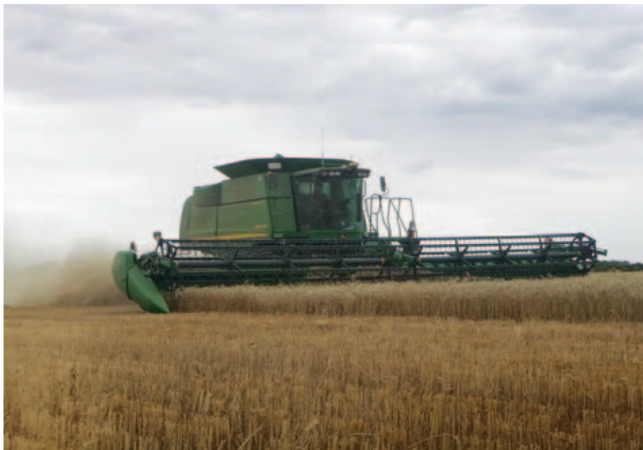
THE NIELDS’ MAIN HEADER FITS THEIR CTF SYSTEM AND USES THE PERMANENT WHEEL TRACKS LIKE THE REST OF THEIR MACHINERY.
