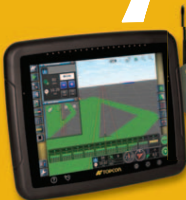
System 350 for steer-ready vehicles. X30 console with AGI-3 receiver/steering controller.
