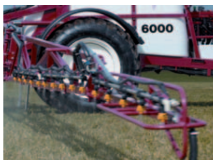
OPERATING THE RIGHT NOZZLES AT THE CORRECT PRESSURE IS THE FIRST STEP TOWARDS REDUCING THE RISK OF OFF-SITE DAMAGE FROM SPRAY DRIFT.
