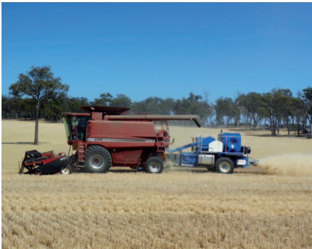
DEVICES LIKE THE HARRINGTON SEED DESTROYER [PICTURED] AND CHAFF CARTS CAN MINIMISE HARVEST-TIME RENEWAL OF THE WEED SEED BANK. PHOTO COURTESY GRDC.
