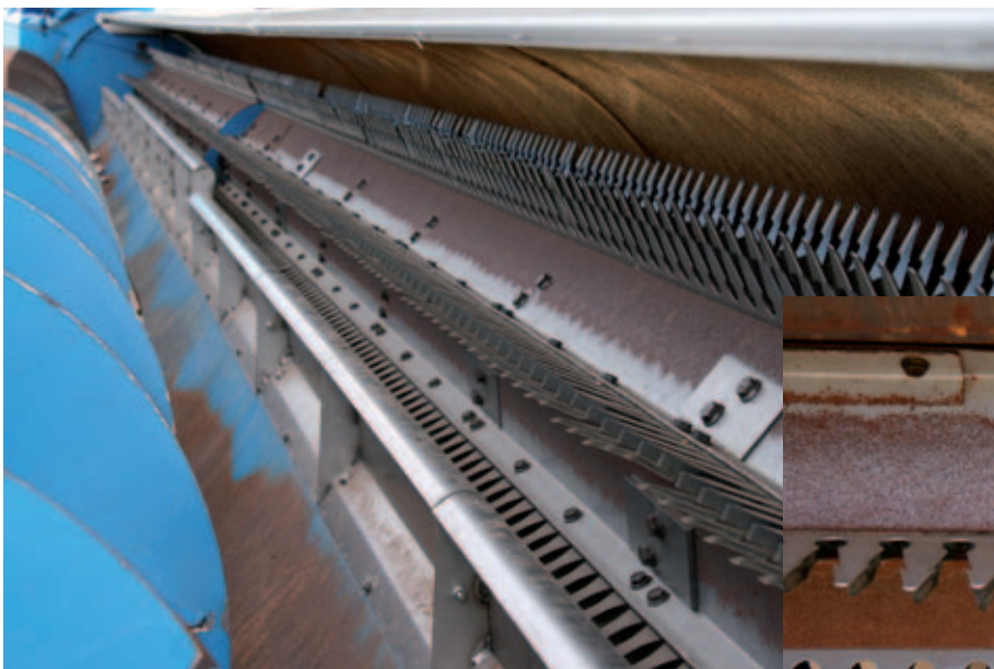
THE 'BUSINESS END' OF A STRIPPER FRONT, IN WHICH 'STRIPPING FINGERS' STRIP GRAIN FROM THE CROP. THIS MEANS MUCH OF THE GRAIN IS THRESHED BY THE HEADER, SO THE MATERIAL ENTERING THE COMBINE IS MOSTLY GRAIN, CHAFF AND LEAF, WITH MOST OF THE STRAW LEFT IN THE PADDOCK. RIGHT: A CLOSE VIEW OF TWO ROWS OF STRIPPING FINGERS.
