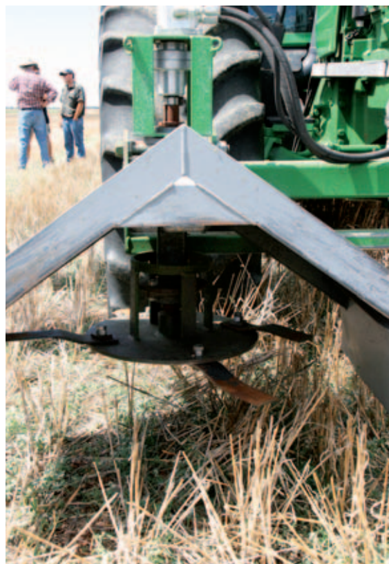
A CLOSE VIEW OF A SLASHER FITTED IN FRONT OF A HEADER WHEEL TO AVOID STRAW BEING ROLLED ONTO THE SOIL SURFACE WHERE IT COULD CAUSE PROBLEMS AT SEEDING TIME.
