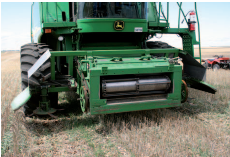
THIS HEADER, WHICH USUALLY CARRIES A STRIPPER FRONT, HAS BEEN FITTED WITH SLASHERS AHEAD OF THE WHEELS SO THEY DO NOT ROLL LONG STRAW ONTO THE SOIL SURFACE.
