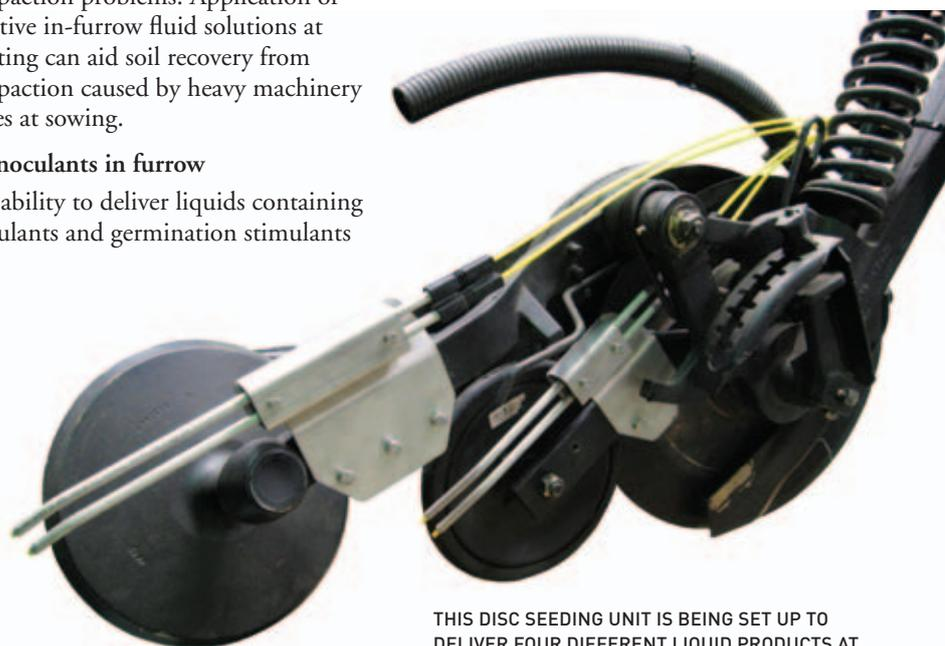
THIS DISC SEEDING UNIT IS BEING SET UP TO DELIVER FOUR DIFFERENT LIQUID PRODUCTS AT DIFFERENT DEPTHS DURING THE SEEDING PASS.
