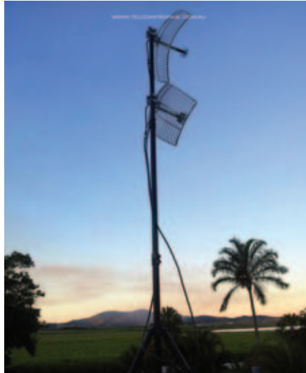
THE PARABOLIC 4G ANTENNAE ABOVE LOOK QUITE DIFFERENT FROM THE 3G ANTENNAE [LOWER RIGHT] AND HAVE VERY DIFFERENT PERFORMANCE CHARACTERISTICS. ABOVE RIGHT IS AN NBN ANTENNA WITH A MODEM PLACED ON IT.
