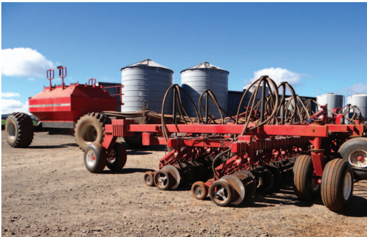
ANDREW'S NEW DISC SEEDER IS MAKING IT POSSIBLE FOR HIM TO REDUCE HIS ROW SPACING AND COMPLETE HIS SOWING PROGRAM IN LESS WORKING HOURS THAN WITH A TINED MACHINE, THOUGH DAMP CONDITIONS CAN HOLD UP SEEDING WITH THE DISC.
