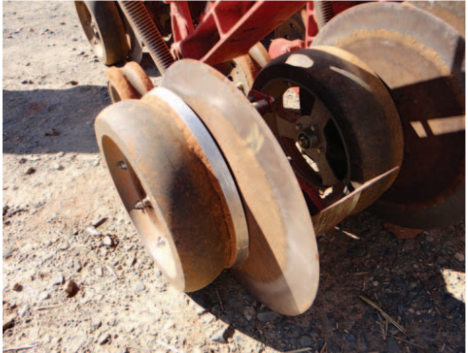
THE DISC SCRAPERS HAVE BEEN MODIFIED TO HANDLE THE CONDITIONS ON SULBY FARM AND NOW WORK WELL. MODIFIED SCRAPERS WILL BE FITTED TO TWO OTHER RAZR DISCS OWNED BY OTHER MID NORTH FARMERS.
