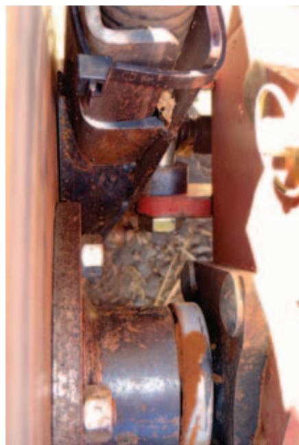
MODIFICATIONS TO THE ORIGINAL SEED BOOTS ON THE RAZR DISC HAVE SIGNIFICANTLY IMPROVED TRASH CLEARANCE.
