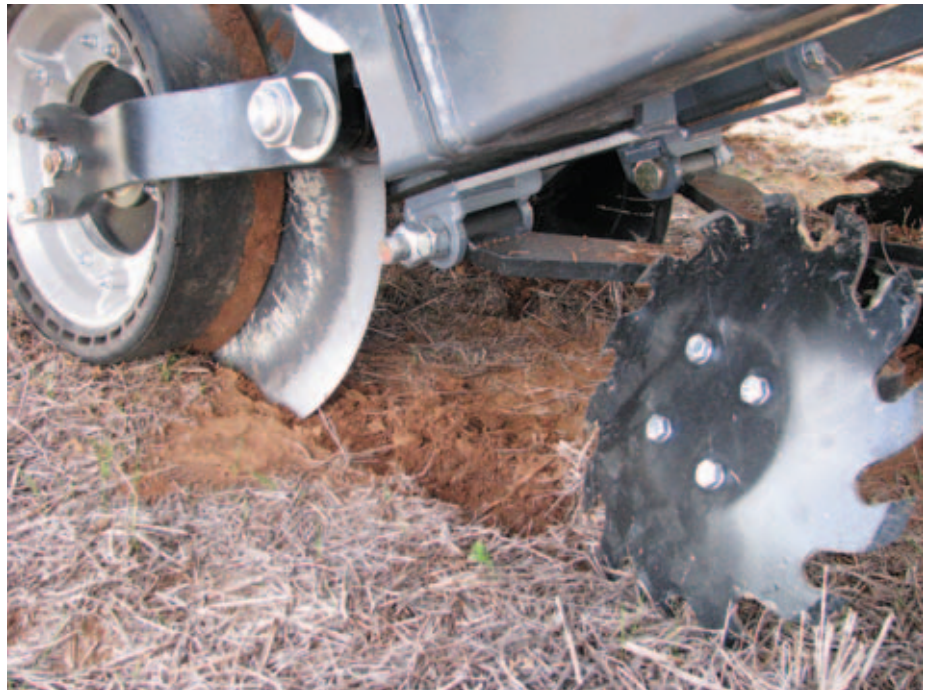
AN NDF SEEDING MODULE WITH RESIDUE MANAGER FITTED.
