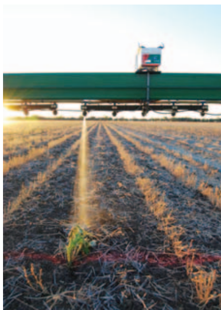
THIS IMAGE LEAVES NO DOUBT ABOUT THE 'SPOT SPRAY' NATURE OF THIS TECHNOLOGY.
