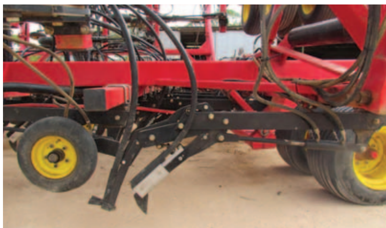
THE DUAL TINE SET UP OF THE SEED HAWK IS QUITE DISTINCTIVE.
