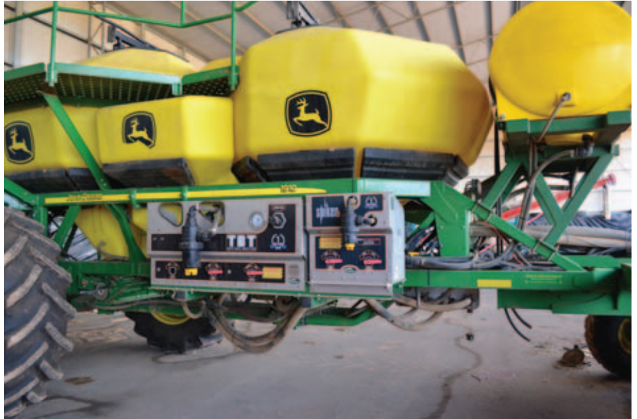
THE CONTROL PANEL OF THE SPIKER SYSTEM; AN IMPORTANT PART OF THE LUSHES' LIQUID DELIVERY SYSTEM.
