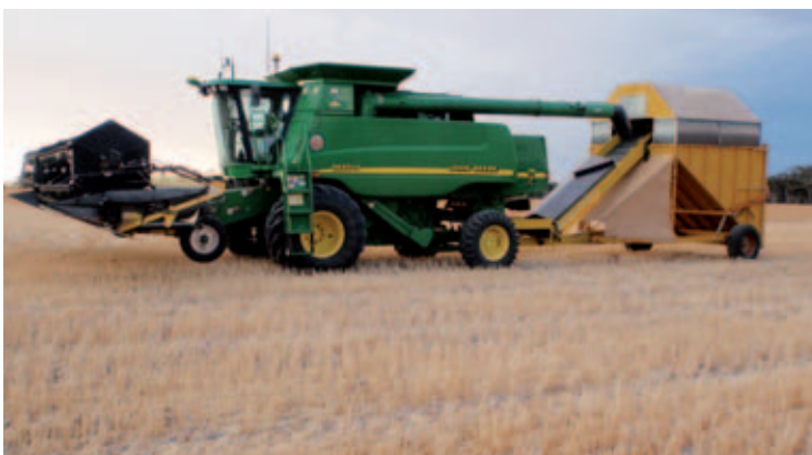
ABOVE: THE ELEVATOR CHAFF DELIVERY SYSTEM SET UP ON LANCE'S FIRST CHAFF CART. RIGHT: LANCE'S NEW CHAFF CART DURING THE 2010 HARVEST. (PHOTOS COURTESY SANDY TURTON.)
