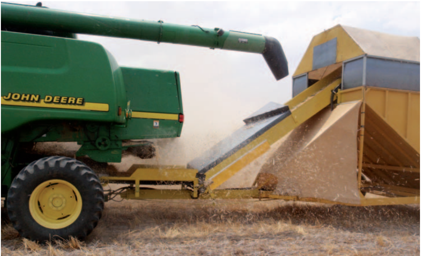
ABOVE: THE ELEVATOR CHAFF DELIVERY SYSTEM SET UP ON LANCE'S FIRST CHAFF CART. RIGHT: LANCE'S NEW CHAFF CART DURING THE 2010 HARVEST. (PHOTOS COURTESY SANDY TURTON.)
