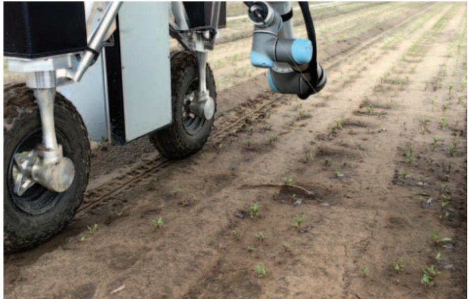
TARGETED SPOT SPRAYING. FITTED ARMS PRECISELY TARGET INDIVIDUAL WEEDS TO MINIMISE HERBICIDE VOLUME.
