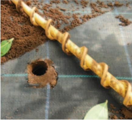
INSTALLING ONE OF THE NEW-GENERATION PROBES IS AS SIMPLE AS POSITIONING THE STABILISING TRIPOD AND DRILLING A HOLE WITH THE TAPERED AUGER.
