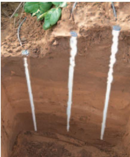
THIS EXCAVATION HAS EXPOSED THE FULL LENGTH OF THREE OF THE NEW-GENERATION TAPERED PROBES AT A DEMONSTRATION SITE. NOTE THE LACK OF SOIL DISTURBANCE AROUND THE PROBES.
