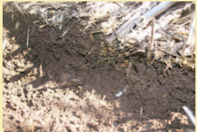
FIGURE 2: DIGGING AWAY THE SOIL ON ONE SIDE OF THE UHP CUT SHOWED THREE KEY FEATURES: HAIR-PINNING WAS VIRTUALLY ELIMINATED, STRAW UP TO EIGHT LAYERS THICK WAS CLEANLY CUT, AND THERE WAS NO OBVIOUS STRUCTURAL DAMAGE TO THE SOIL OR SMEARING OF THE SIDE WALL.
