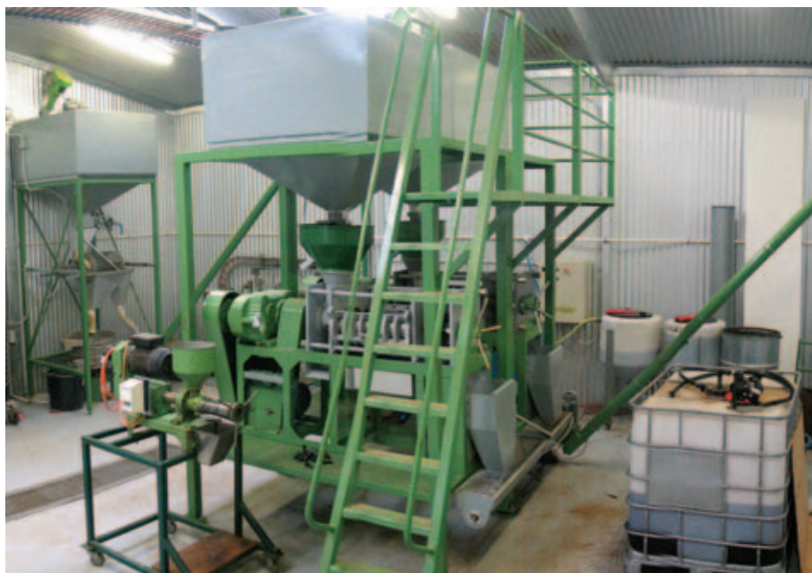
THIS OILSEED PRESS, IN A FARM SHED ON STEVE HOBBS’ KANIVA PROPERTY, IS THE FIRST STEP IN CONVERTING HIS MUSTARD SEED TO FUEL AND STOCK FEED.
