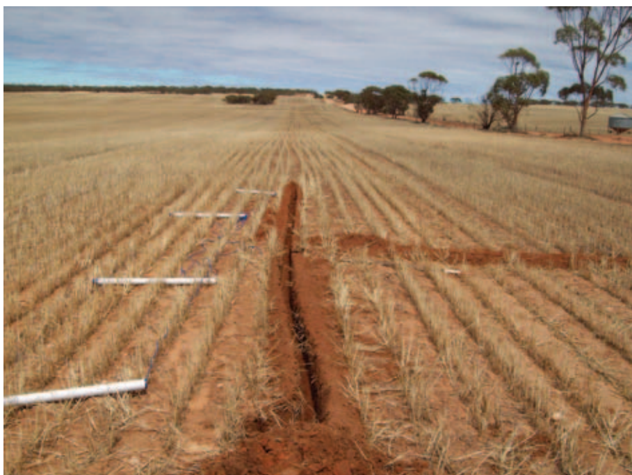
PREPARING TO INSTALL A LINKED SERIES OF MOISTURE PROBES [LEFT] IN A TRIAL SITUATION.
