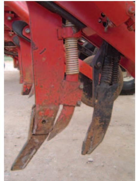
A NARROW POINT AND DEEP BANDING BOOT ALLOWS FOR SEED AND FERTILISER TO BE SEPARATED ENSURING FERTILISER IS LESS LIKELY TO CAUSE TOXICITY.
