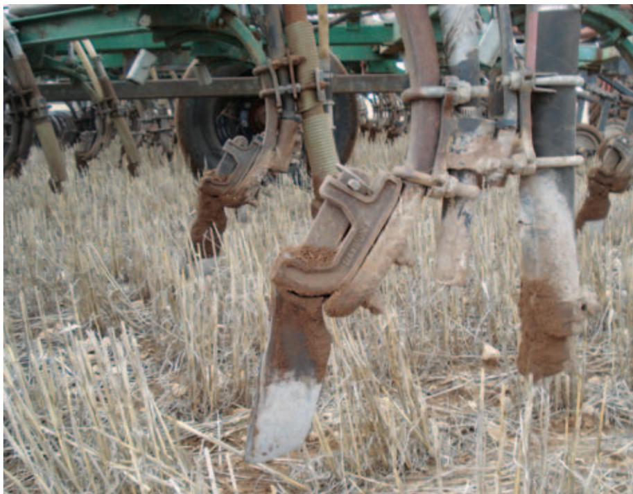
A TYNE MACHINE REMAINS A GOOD OPTION FOR MANY GROWERS. TO ENSURE OPTIMAL PERFORMANCE IT IS IMPORTANT TO CHECK SEED DELIVERY CALIBRATION, INCLUDING SEED DELIVERY ACROSS THE TOOL BAR, AHEAD OF SEEDING EACH YEAR AND PERIODICALLY CHECK FOR BLOCKED BOOTS AND DISTRIBUTION HEADS.
