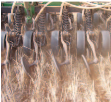
ROW SPACING AND MACHINE WEIGHT BOTH INFLUENCE THE ABILITY TO PENETRATE AND KEEP DISCS IN THE SOIL.
