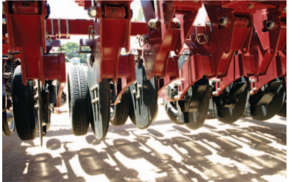
DISC DIAMETER, SHARPNESS AND OPERATING DEPTH ALL INFLUENCE THE PERFORMANCE OF DISC SEEDERS AND GETTING THE BEST RESULTS REQUIRES CLOSE ATTENTION TO DETAIL.
