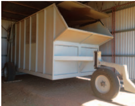
CAPTURING WEED SEEDS WITH A HOMEMADE CHAFF CART HAS REDUCED THE PFITZNER'S WEED BURDEN BY 70%.
