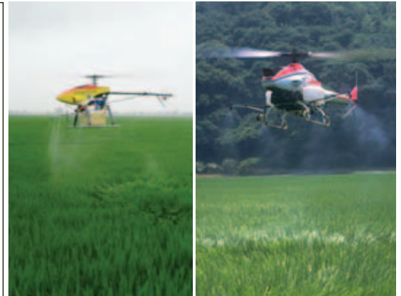
ABOVE: WHILE MUCH OF THE WORK WITH RPAs HAS FOCUSED ON DATA CAPTURE, THEY CAN ALSO BE USED FOR PADDOCK SPRAYING, WHICH OPENS THE WAY TO TARGET CHEMICALS ON AREAS WITH HIGH WEED OR DISEASE POPULATIONS.
