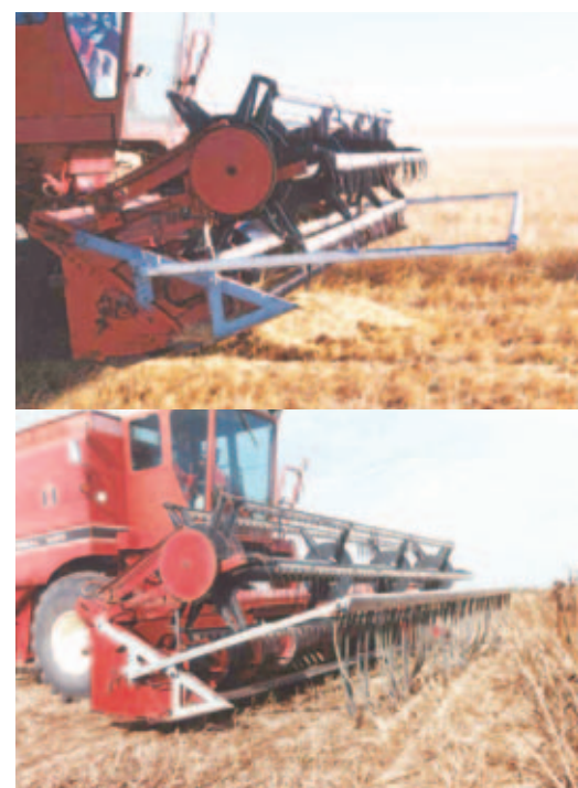
FIG. 1: RIGID DISLODGER BAR (TOP) FOR CEREALS AND WITH ADD-ON DANGLING BELTS (ABOVE) FOR FABA BEAN.
