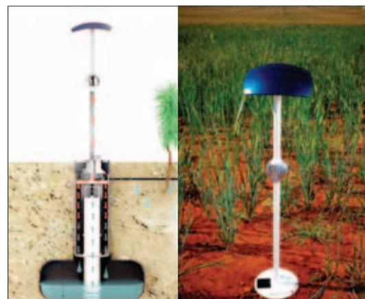
ABOVE LEFT: A SCHEMATIC DIAGRAM OF A SELF-CONTAINED AIRDROP SYSTEM. HOT AIR DRIVEN INTO THE VERTICAL TUBES BY THE TURBINE ON THE STEM IS COOLED AND RELEASES MOISTURE, WHICH DROPS INTO THE RESERVOIR BELOW, FROM WHERE IT IS PUMPED TO NEARBY PLANTS.
