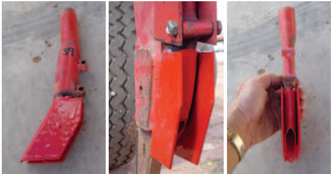
AT RIGHT (LEFT TO RIGHT): A SIDE VIEW OF ONE OF THE WINGED FERTILISER BOOTS DEVELOPED TO REDUCE TRASH BLOCKAGES AND IMPROVE FERTILISER FLOW; A CLOSE UP OF A TINE FITTED WITH A WINGED FERTILISER BOOT; A REAR VIEW OF ONE OF THE WINGED FERTILISER BOOTS FITTED TO THE FERTILISER TUBES ON ANDREW CASS'S CONSERVA PAK SEEDER.
