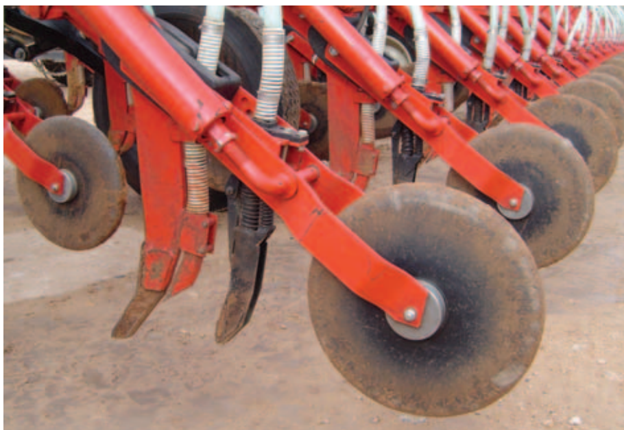
A TINE ASSEMBLY ON THE SEEDER BEFORE ADDITION OF THE WINGED FERTILISER BOOTS ANDREW HAD FITTED TO PREVENT TRASH WRAPPING AROUND THE POINT AND BLOCKING THE TUBE.
