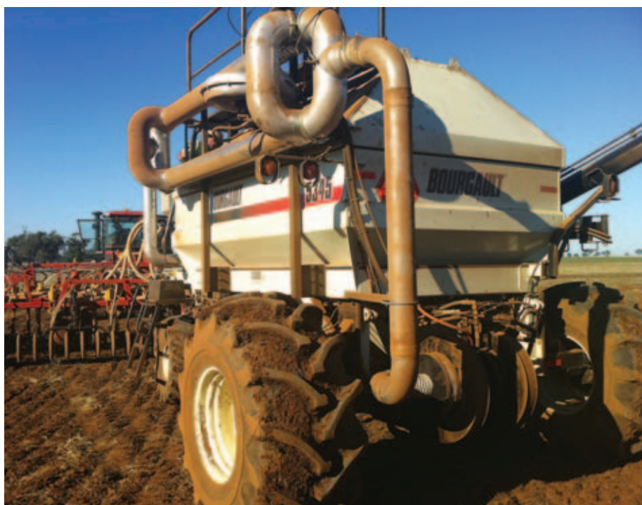
A BOURGAULT AIR-SEEDER FITTED WITH BIO-AGTIVE EMISSIONS TECHNOLOGY THAT INJECTS TRACTOR ENGINE EMISSIONS INTO THE SOIL.
