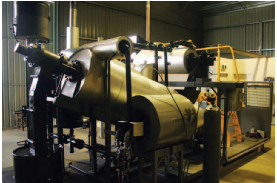
THE ELMORE BIOCHAR PRODUCTION PLANT HAS A FEEDSTOCK CAPACITY OF 200 KG/HR AND CAN PRODUCE 80 KG/HR OF BIOCHAR.
