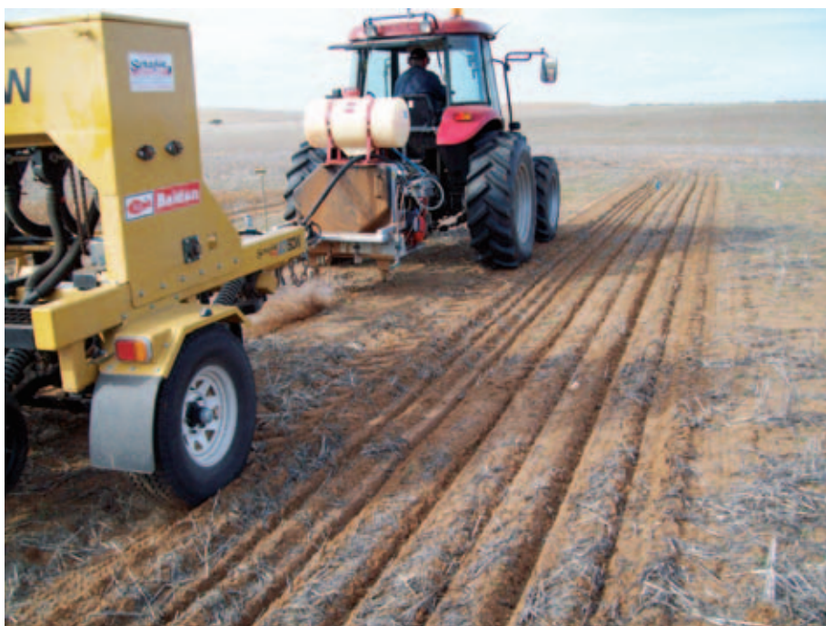
FIGURE 5: INJECTING FUNGICIDE IN FRONT OF DISC-SEEDED WHEAT AT KAROONDA DID NOT IMPROVE RHIZOCTONIA CONTROL COMPARED TO FUNGICIDE APPLIED AS A SEED DRESSING. HOWEVER, THE AQUA-BAND DELIVERY MECHANISM CAN BE SIGNIFICANTLY IMPROVED THROUGH USE OF A GROUND ENGAGEMENT TOOL SUCH AS A PARALLELOGRAM, BENEFITS MAY BE GAINED FROM THIS TYPE OF APPLICATION METHOD IN THE FUTURE.
