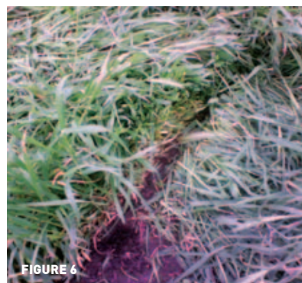
FIGURE 6 WEEDY BIOMASS SLASHED WITH 10/1000” (0.254 MM) NOZZLE AT 50,000 PSI (3,447 BAR).
