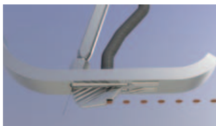
FIGURE 1: AN AQUA-TILL CONCEPT DESIGN USING A NOZZLE EMBEDDED AT A 150 FORWARD RAKE ANGLE IN A SKI WITH A KEEL-STYLED SEED DELIVERY MECHANISM. THIS CONCEPT MAY HAVE PROMISE FOR SEEDING INTO WET, SOFT SOILS WITH HEAVY STUBBLE COVER.
