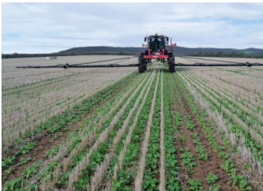
THE DOUDLES' SELF-PROPELLED SPRAYER OPERATING ON PERMANENT CTF WHEEL TRACKS.
