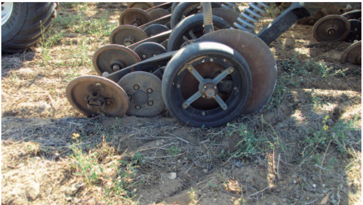
TYRE SHAPE AND COMPOSITION HAVE A BIG IMPACT ON PRESS WHEEL PERFORMANCE, SO IT IS IMPORTANT TO CHOOSE THE RIGHT TYRE FOR THE CONDITIONS.
