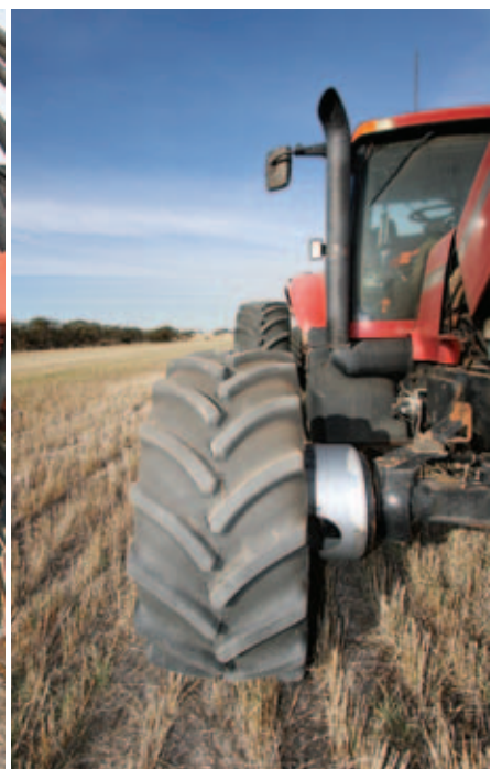
ABOVE RIGHT: WES’S TRACTOR WAS MODIFIED TO FIT THE STANDARD TRACK WIDTH BY CUTTING THROUGH THE FRONT AXLE AND WELDING IN A SECTION OF PIPE TO PUT THE FRONT WHEELS ON THREE-METRE CENTRES.
