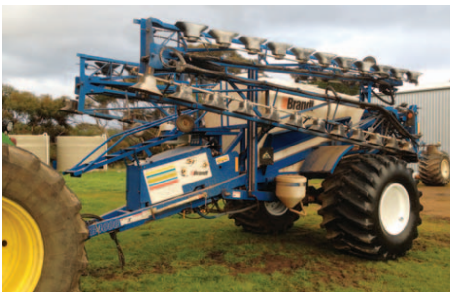
SPRAYING IS AN IMPORTANT PART OF CROP MANAGEMENT FOR THE STANTONS, WHO HAVE TRIALLED A VARIETY OF DIFFERENT SPRAY UNITS, FROM A SELF-PROPELLED SPRAYER (TOP) TO THEIR CURRENT MACHINE, A TRAILED BRANDT SB4000 (MID AND BOTTOM) WITH A 30-METRE BOOM FITTED WITH SHIELDED NOZZLES TO MAXIMISE CONTROL OF THE SPRAY PATTERN.
