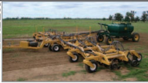
**High quality, low maintenance, heavily constructed No-Till Seeder, sizes ranging from 20ft-66ft. Fitted with New Baldan 20" single disc row units.**
