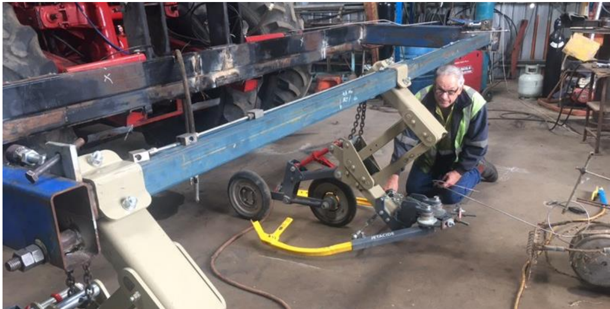
Figure 7: Graham working on the parallelogram inspired engagement tool. The basic design has been modified to accommodate the grains application (vertical nozzle) and an alternative application for cotton ratoon control (horizontal nozzle)
